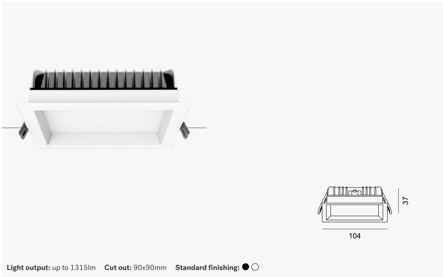
**Light output:** up to 1315lm   **Cut out:** 90x90mm   **Standard finishing:** ● ○
